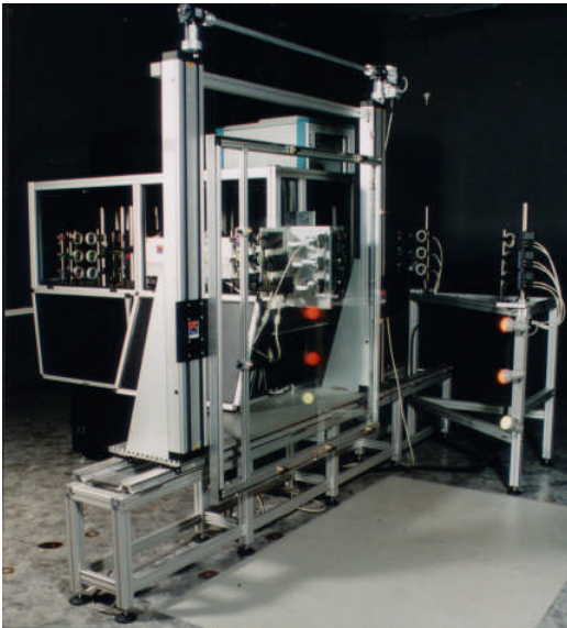
Fig.2 The first RGB Pulsed-Laser Holographic Printer made by Geola in 2001
